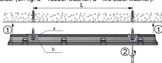
3.1. Suspended installation. Drill installation holes in luminaire's body, L – distance between holes: (on fig. a – M6 steel washer; b - rubber washer; c- M6 nut).
